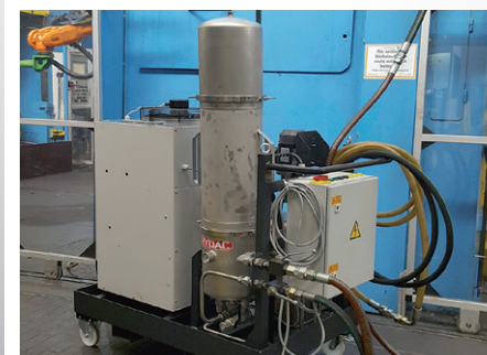
Unit for the removal of oil degradation products (VEU-F), either with a plate heat exchanger or a compressor cooler
