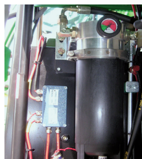
Filters with superabsorbers (Aquamicron®)
