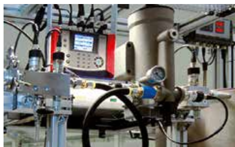
HYDAC laboratory and test bench to determine water separation efficiency
