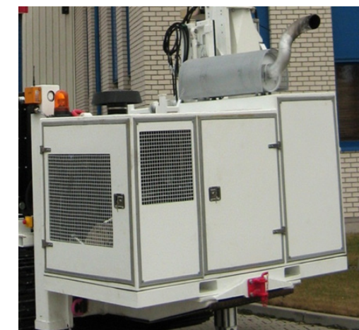
Piggyback power unit for crawler drill rig
