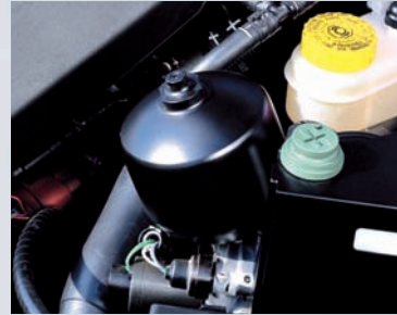
Lightweight diaphragm accumulator for energy storage in the automatic gear shift system
