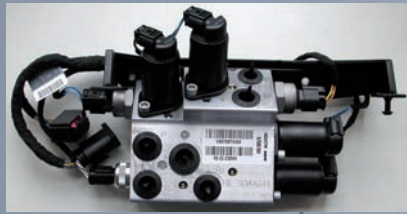
Electro-hydraulic systems for active roll stabilization for top range car
