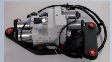
Electro-hydraulic systems for active roll stabilization for SUV
