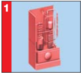
1 Fluid panel consisting of Hydraulic Power Unit, Hydraulic Control, Filtration, Pneumatics, Central Lubrication and FWKS Cooling System.
