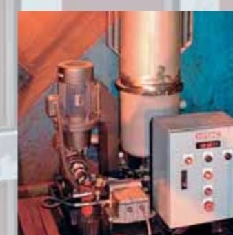
OLF Off-line Filtration with ContaminationSensor CS 2000.
