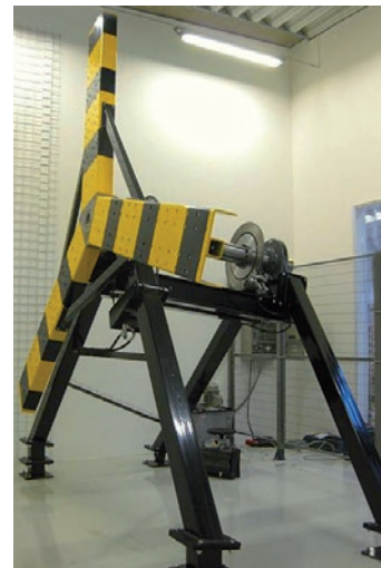
Rotation test rig for components, e.g. bladder and piston accumulators
