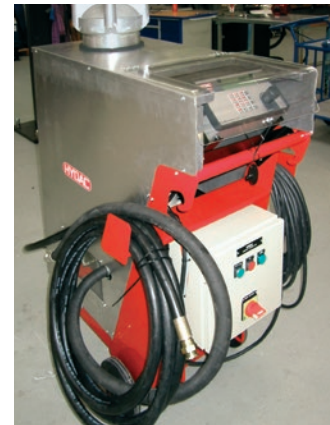
Filter transfer unit for filling and cleaning hydraulic and lubrication systems, including particle counter and heater
