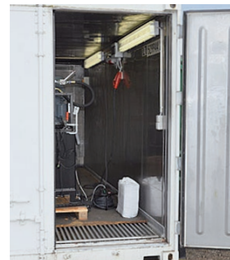
Test rig for low temperature testing, e.g. water glycol systems and oil supply
