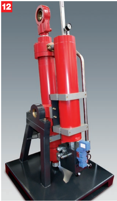
Cylinder for pitch adjustment with integrated linear position system, subplate-mounted control block with control valve and piston accumulator for emergency function
