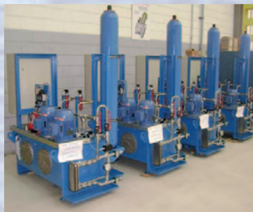
Power units for turbine controller
