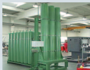
Accumulators for emergency shut-off of spherical / butterfly valve
