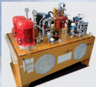
Hydraulic turbine controller
