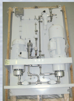
Start lift system (high pressure)
