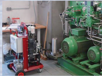
Mobile unit for dewatering, degassing and filtration: FluidAquaMobil FAM
